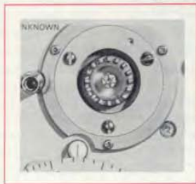
Figure 1. Type 1606-B RF Bridge. Inset shows GR900® adaptor in place.
