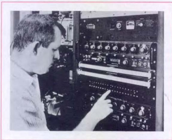
Figure 1. Type 1163 synthesizer under control of 40-channel program unit. Additional frequencies are available in second 40-channel unit.
